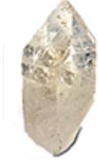
In the 1920s, scientists discovered that quartz crystals could keep even more accurate time than a pendulum. Quartz is a type of crystal that looks like glass. When you apply voltage, or electricity, and pressure, the quartz crystal vibrates at a very constant frequency. This vibration moves the clock's hands very precisely. Many of the clocks and watches we use today are made using quartz.
